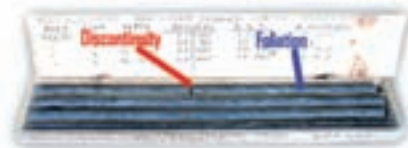
Diagram 3: a massive rock core that was misinterpreted as being easy to excavate
